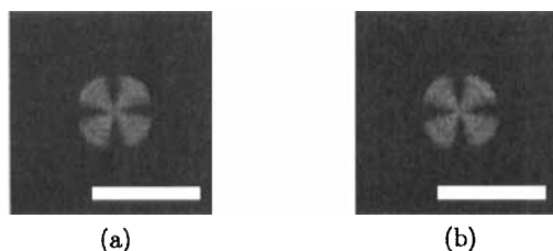
Figure 1 Polarizing microscope images of a Sm-A spherical domain without defects (a) before electric field is switched on and (b) after electric field is switched on. Electric field strength is 1.0 \text{ V}/\mu\text{m} . The bars indicate 50 \mu\text{m} .
